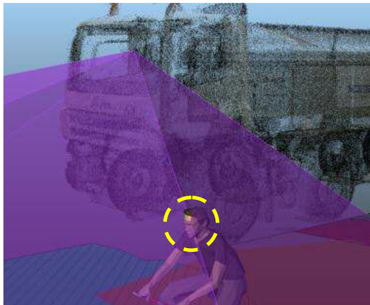
Figure 3-4: The 1.5m tall cyclist in position 9 showing the small area of forehead that is potentially visible in the lower nearside corner of the windscreen of the DAF Tipper
